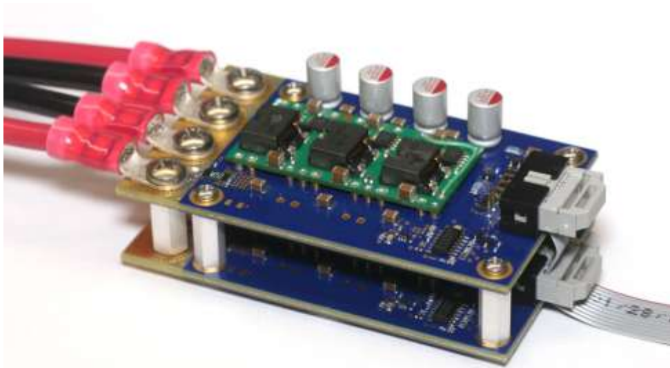
2ea Drivers Stacked for 100A Max Output Current
