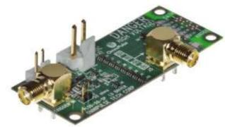
Mounting holes are supplied which accept the most common laser diode packages (5.6 mm, 9 mm, TO-18, TO-5 and TO-52). This allows the light to exit normal to the driver; however, edge mounting of these laser diodes can also be accommodated.
