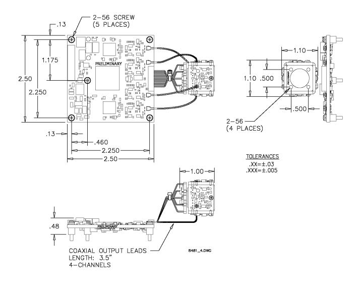
Sensor Assembly Dimensions are in inches.
