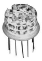
The **Model 755** hybrid eyesafe laser rangefinder receiver is designed for laser rangefinding/surveying equipment. Because of the compact construction (Modified TO-8 header) and the PCB mounting capability, it is ideal for miniature applications. Fast recovery from  $T_0$  overload allows ranging to close objects without compromising long range performance. The incorporation of an InGaAs APD gives very high sensitivity.
