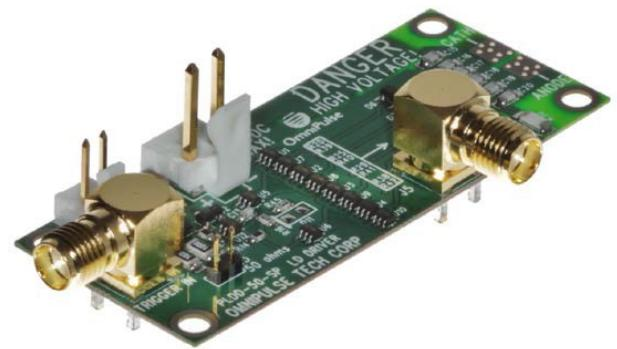
The PLDD-50-SP is a compact all solid-state, pulsed current source designed to drive single or multichip laser diodes. The unit features a peak current of 50A. The pulse repetition frequency can be varied from single shot to 15kHz at maximum current. Higher repetition frequency is possible at lower current, see graph on next page.
